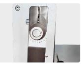
Punch 700 models come equipped with eccentric shafts. This feature allows the dies to be sharpened a few times.
