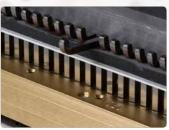
QSA (Quick Size Adjustment) technology allows the quick cancellation of punching pins without having to remove the die.<sup>(1)</sup>
