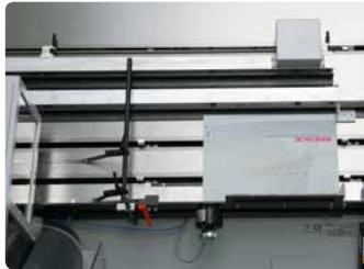
In-feed triggered by a magic eye. The delivery system accurately feeds the product into the punching station.
